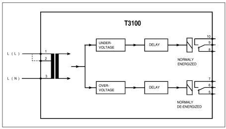
Connection Diagram. Relay shown de-energized.
